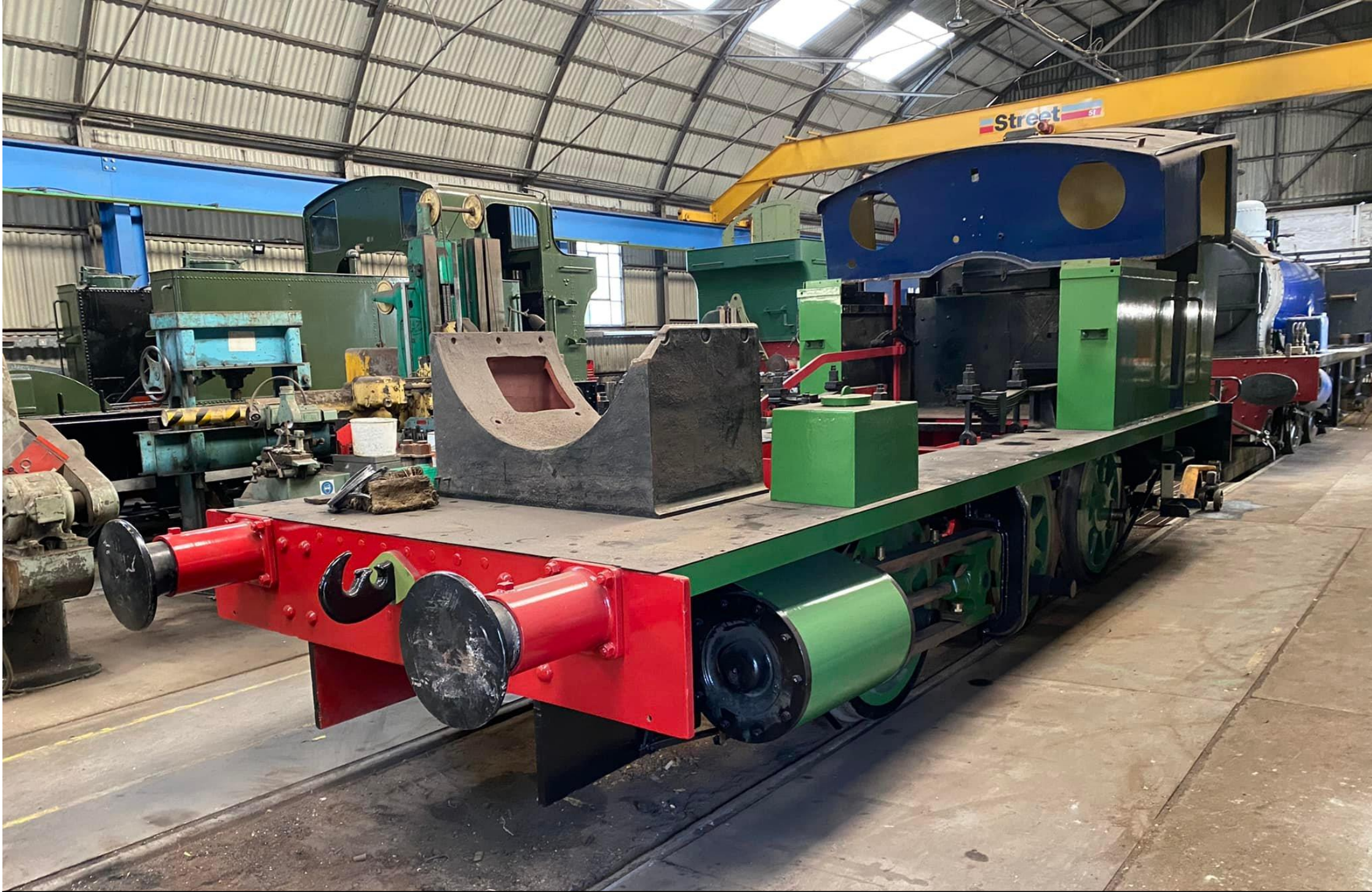
Steam Department Andre Barclay 2074 Llantarnam Abbey undergoing restoration at West Somerset Restoration, Williton
